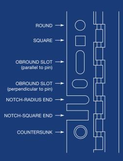
**2.** Bending — Fitting a hinge into the space allotted for it may require various types of bending. We do all bending in our secondary department. Variations include:
